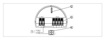
Electronics and connection compartment, single chamber housing (example)
